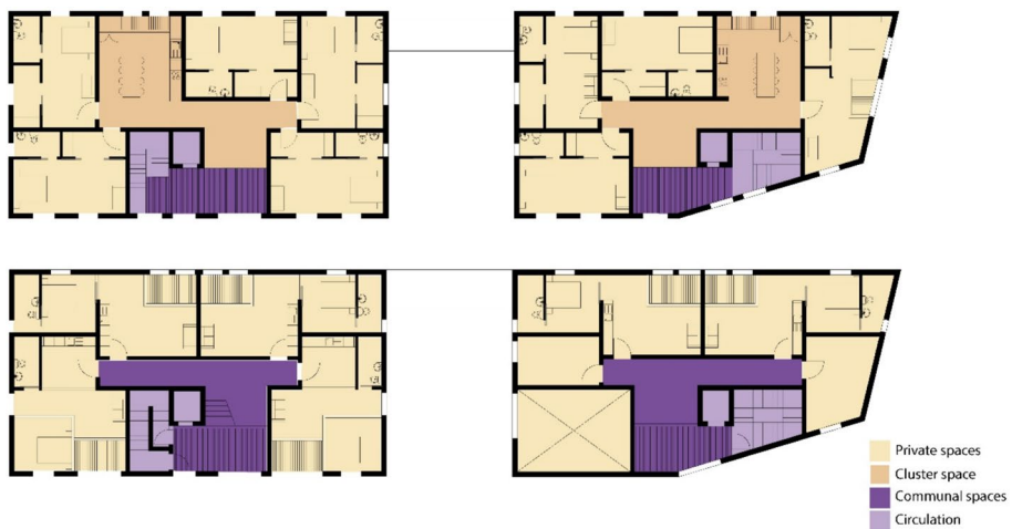
Fig. 8 On the top: typical floor plan of cluster units, on the bottom: typical floor plan of conventional units.
