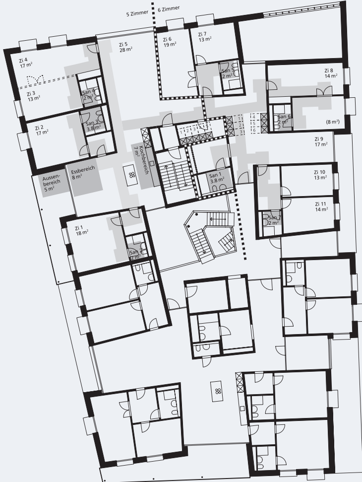
2.4 Haus A cluster typology, cited as an exemplary floor plan for “Flexible Forms of Living” in the federal design guidelines WBS, 2015
